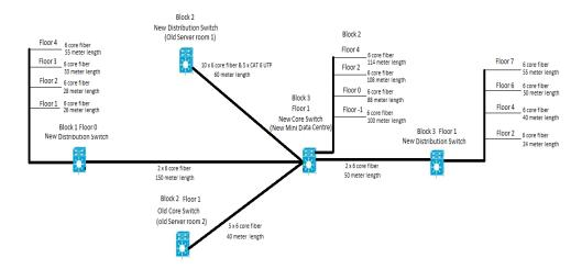
Figure 1 - Fibre connections from new backbone switch to existing core switch and floor switches
